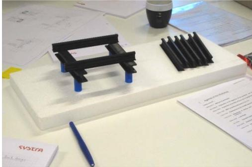
3D-printed mock-up of an early SP1 track concept
